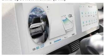
Blind-Spot View Monitor displays video of the blind-spot view for a safe lane change. When operating the turn signal switch, BVM displays video of the blind-spot view for the direction indicated.
