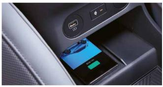
The high speed wireless charger incorporates a cooling function that prevents the smartphone from overheating for added safety and convenience.
