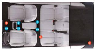
Front: 2 USB chargers, 1 USB port for data support, 1 power outlet.
